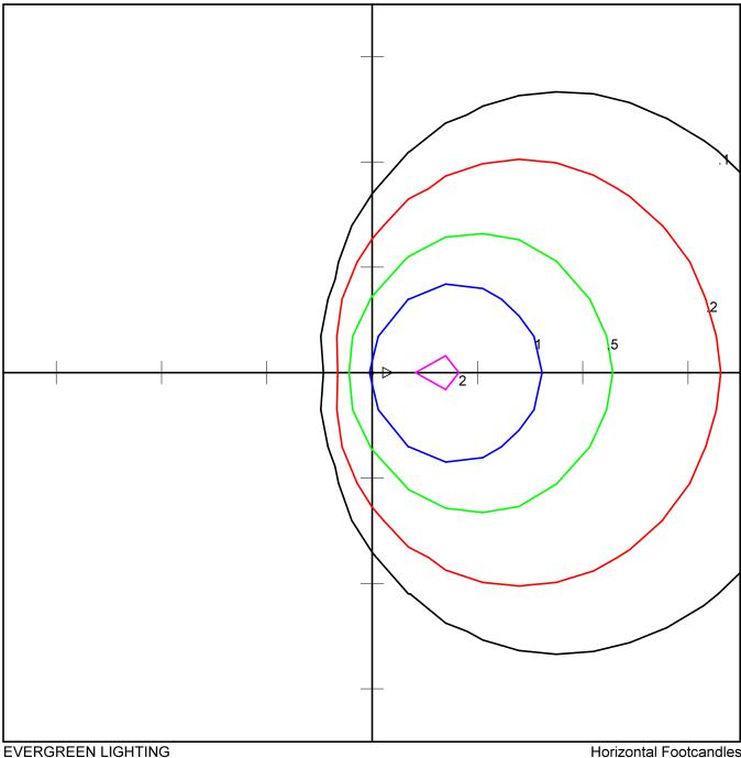
EVERGREEN LIGHTING MO-16-24LED WALL SERIES, WHITE HR ACRYLIC LENS (2) ALTA PN110B-11" LED BOARDS Horizontal Footcandles
