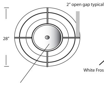
**Bottom White Frosted** Acrylic regress upward 2" White Frosted acrylic 4- Aluminum square bar @ 90 degrees on acrylic rings
