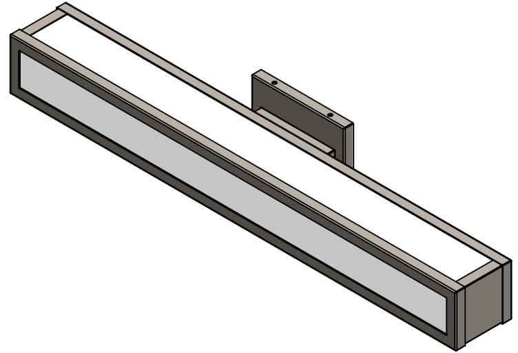
PLATES SPOT WELDED TOGETHER
