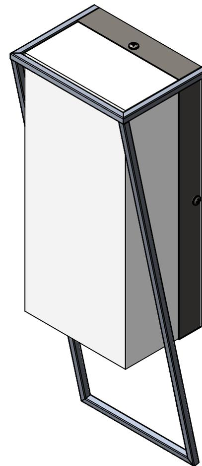
ALL SPOT WELDED TOGETHER INTO ONE PIECE
