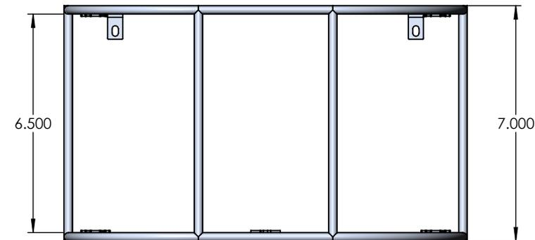
ALL TABS WELDED TOWARDS THE INSIDE OF THE WIRE FRAME
