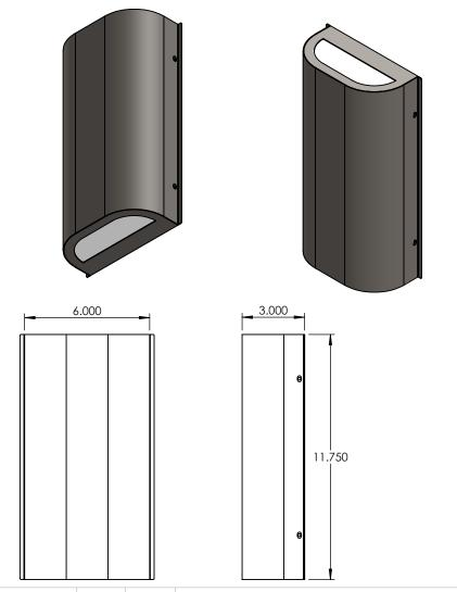
UNLESS OTHERWISE SPECIFIED: NAME DATE DRAWN DIMENSIONS ARE IN INCHES TOLERANCES: CHECKED FRACTIONAL± .003 ANGULAR: MACH±.01 BEND ± ENG APPR. TWO PLACE DECIMAL ± THREE PLACE DECIMAL ±.001 MFG APPR. Q.A. INTERPRET GEOMETRIC TOLERANCING PER: COMMENTS: MATERIAL
