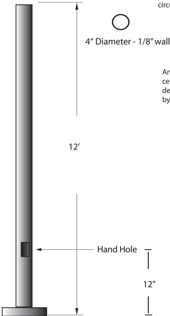
Pole is welded circumferentially to base.
