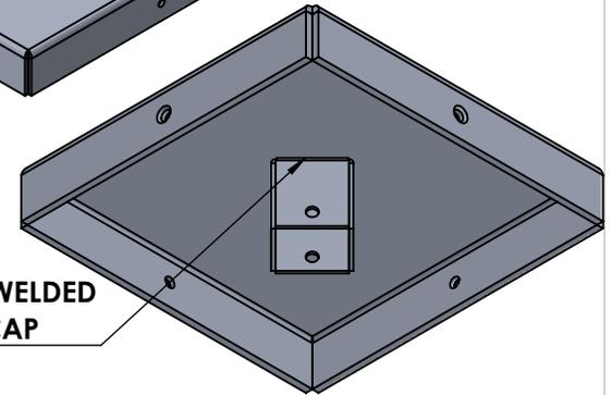
**TUBE BRACKET WELDED TO INNER CAP**
