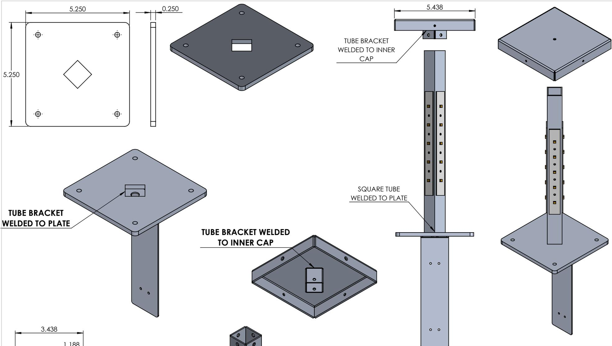
TUBE BRACKET WELDED TO PLATE
