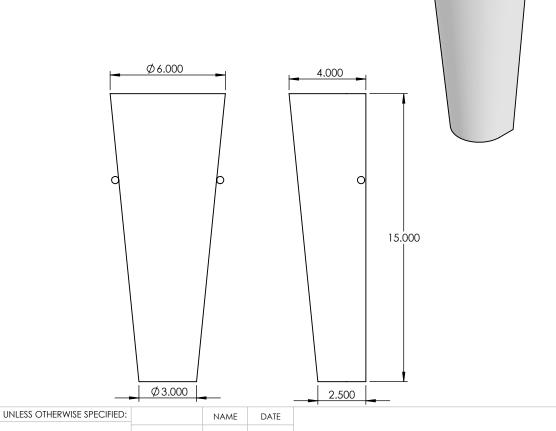
DRAWN DIMENSIONS ARE IN INCHES TOLERANCES: TITLE: CHECKED FRACTIONAL± .003 ANGULAR: MACH±.01 BEND ± ENG APPR. TWO PLACE DECIMAL ± TRPD-SC-15-15W-MW-WF-DIM-40K THREE PLACE DECIMAL ±.001 MFG APPR. Q.A. INTERPRET GEOMETRIC TOLERANCING PER: COMMENTS: MATERIAL SIZE DWG. NO. REV **TICKET 26926** FINISH SCALE: 1:5 WEIGHT: SHEET 1 OF 5 DO NOT SCALE DRAWING
