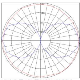
Maximum Candela = 1867.188 Located At Horizontal Angle = 300, Vertical Angle = 90 # 1 - Vertical Plane Through Horizontal Angles (300 - 120) (Through Max. Cd.) # 2 - Horizontal Cone Through Vertical Angle (90) (Through Max. Cd.)
