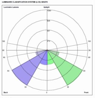
Luminaite Lumens Front: Low-380.5, Medium=1083.1, High=323.0, Very High=5.9 Back: Low=386.9, Medium=1089.5, High=308.0, Very High=5.6 Uplight: Low=1.9, High=9.4
