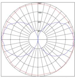
Maximum Candela = 1867.188 Located At Horizontal Angle = 300, Vertical Angle = 90 # 1 - Vertical Plane Through Horizontal Angles (300 - 120) (Through Max. Cd.) # 2 - Horizontal Cone Through Vertical Angle (90) (Through Max. Cd.)
