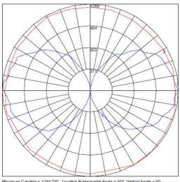
Maximum Candela = 1244.792 Located At Horizontal Angle = 300, Vertical Angle = 90 # 1 - Vertical Plane Through Horizontal Angles (300 - 120) (Through Max. Cd.) # 2 - Horizontal Cone Through Vertical Angle (90) (Through Max. Cd.)
