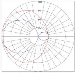
Maximum Candela = 1083.147 Located At Horizontal Angle = 165, Vertical Angle = 100 # 1 - Vertical Plane Through Horizontal Angles (165 - 345) (Through Max. Cd.) # 2 - Horizontal Cone Through Vertical Angle (100) (Through Max. Cd.)
