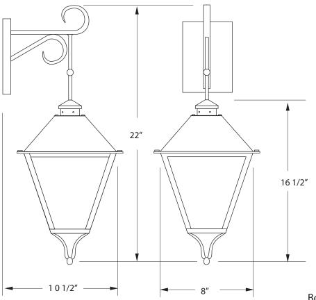
Bottom of the fixture to the center of the canopy is 18 3/4"
