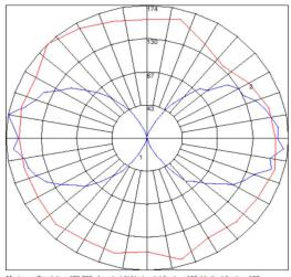
Maximum Candela = 173.739 Located At Horizontal Angle = 135, Vertical Angle = 100 # 1 - Vertical Plane Through Horizontal Angles (135 - 315) (Through Max. Cd.) # 2 - Horizontal Cone Through Vertical Angle (100) (Through Max. Cd.)
