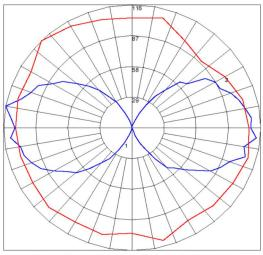
Maximum Candela = 115.826 Located At Horizontal Angle = 135, Vertical Angle = 100 #1 - Vertical Plane Through Horizontal Angles (135 - 315) (Through Max. Cd.) #2 - Horizontal Cone Through Vertical Angle (100) (Through Max. Cd.)
