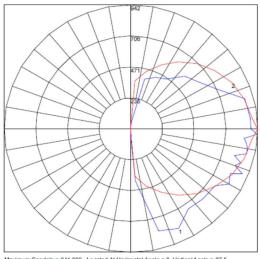
Maximum Candela = 941.869 Located At Horizontal Angle = 0, Vertical Angle = 87.5 # 1 - Vertical Plane Through Horizontal Angles (0 - 180) (Through Max. Cd.) # 2 - Horizontal Cone Through Vertical Angle (87.5) (Through Max. Cd.)
