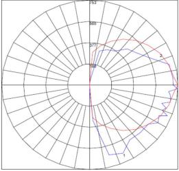
Maximum Candela = 753.335 Located At Horizontal Angle = 0, Vertical Angle = 87.5 # 1 - Vertical Plane Through Horizontal Angles (0 - 180) (Through Max. Cd.) # 2 - Horizontal Cone Through Vertical Angle (87.5) (Through Max. Cd.)
