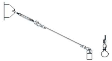
TRB 1/2" 4' Cable Support TRB 3/4" 4' Cable Support
